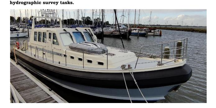
Length overall 16,40 m Width overall 5,26 m Draft app. 1,20 m Clearance height 3.55 m 24 t Displacement 4.0001 Capacity fuel tanks 1.0001 Capacity drinking water tank 4001 Capacity waste water tank
